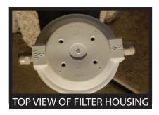
3. The tubing coming from the Reverse Osmosis Post Filter connector needs to be inserted into the side of the housing marked "IN". Firmly press the tubing into the filter-housing cap. You will feel the tubing stop when it is fully inserted. Pull on the tubing gently to ensure that it does not come out and a good connection was made.
